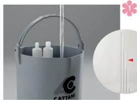
Fill the Cattani Pulse Cleaner with 2.5 litres of ambient temperature water which is halfway between the second and third line of the Pulse Cleaner.
